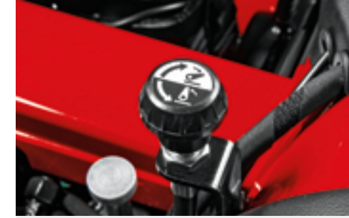
MAXIMUM LIFT HEIGHT SETTING CONTROL Affords greater working precision and protection for implements powered by PTO drive shaft.
