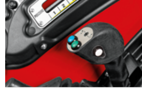
HAND GRIP WITH ELECTRICAL CONTROL BUTTONS Controls for proportional activation of the remote valves.
