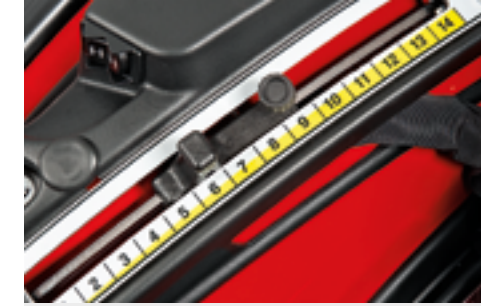
LIFTING WITH POSITION AND DRAFT CONTROL Mixed control device.
