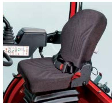
> SIÈGE AVEC SUSPENSION PNEUMATIQUE GRAMMER
